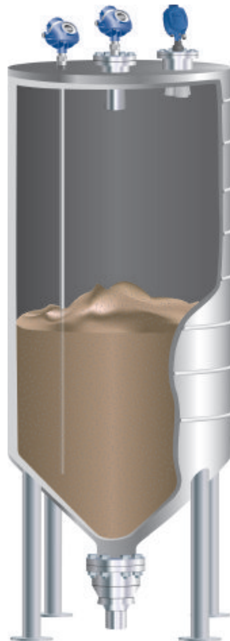
Figure 1: This hypothetical vessel has representations of all three measuring technologies: guided-wave radar, noncontact radar, and acoustic. All graphics courtesy: Emerson Process Management
